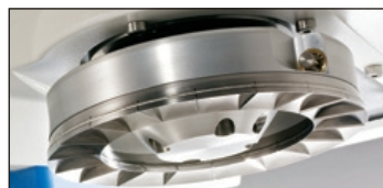
Closed-up View of Vane Lid used for Flow Function Test.
