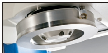
Closed-up View of Wall Friction Lid for wall friction test and density test
